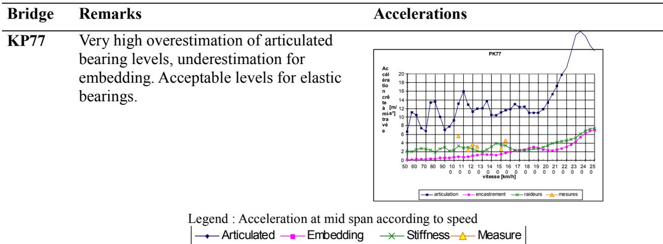
Figure 6: Calculated acceleration / measured acceleration
