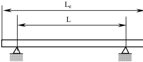
This  $L/L_e$  relationship has little influence on the value of the natural frequency on condition that the length does not exceed 30% of the span.
