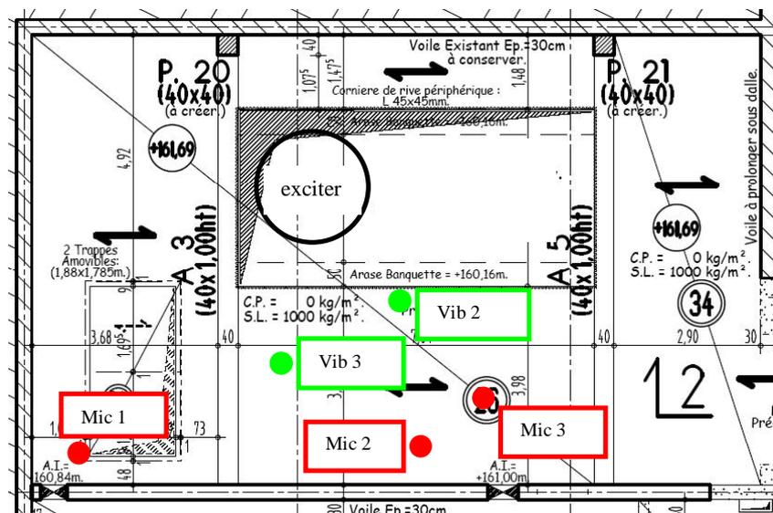
Figure 1. Layout of exciter test room
