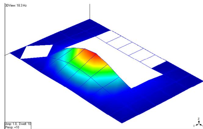
Figure 5. Mode shape of floor in area Vib2, frequency 18.3 Hz damping 1.2 %
