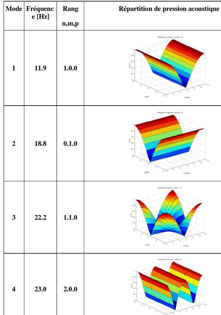
Figure 3. Acoustic mode shapes in test room (calculated).
