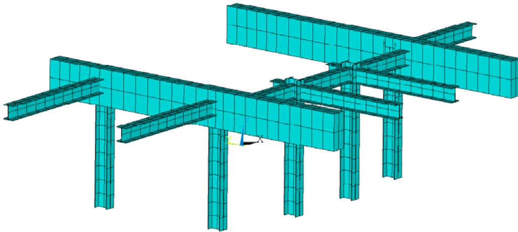
Figure 8. Accepted stiffening solution for laboratory floor.
