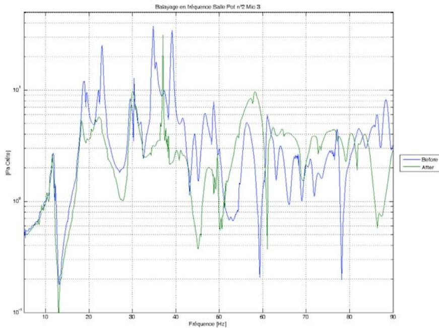
Figure 10. Acoustic pressure at mic 3 during sweep of exciter, before / after implementing Helmholtz resonators
