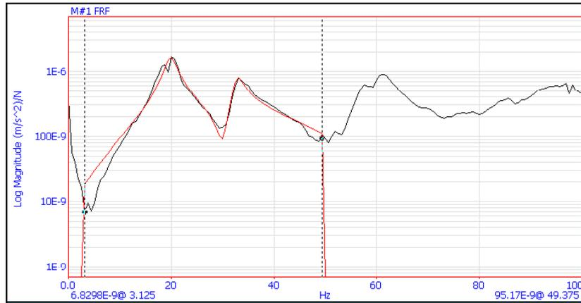
Figure 4. Vertical inductance of floor in area Vib2
