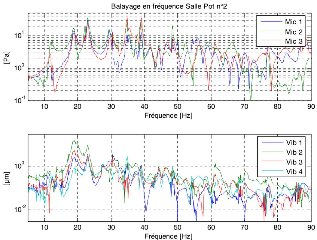
Figure 2. Acoustic pressure in room, and vertical displacement of floor during exciter sweep.
