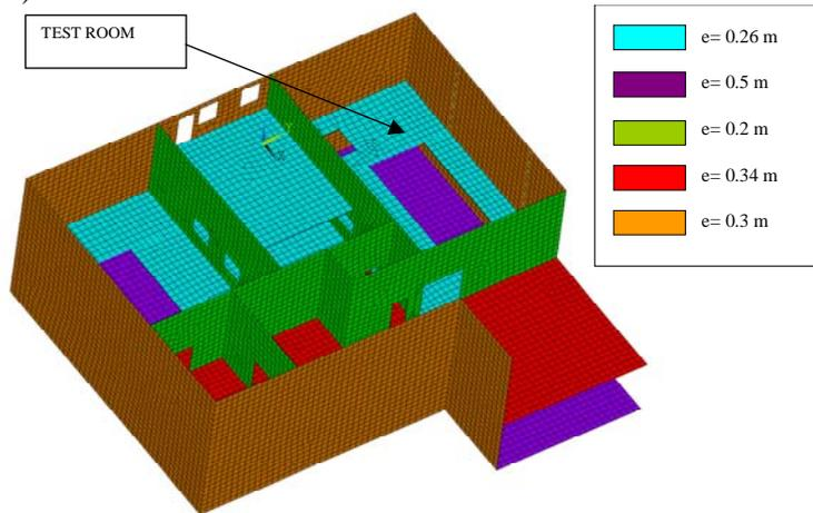
Figure 6. Finite element model (Ansys) of overall structure of laboratory.
