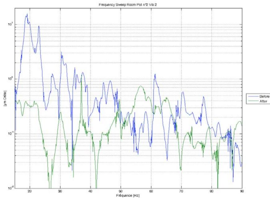
Figure 11. Vibration displacement at vib 2 during sweep of exciter, before / after implementing structural stiffening
