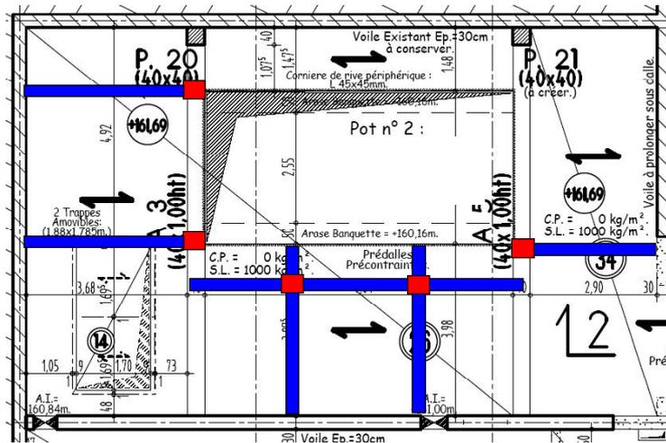
Figure 7. Typical stiffening solution for laboratory floor.
